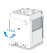
Insert filament spool holder into rear slot of Robo C2 with the taller tab end first. Make sure to insert the spool holder completely inside the printer — not in the small space directly behind the printer's plastic back panel.
