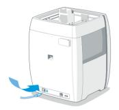
4. Connect power adapter and cable to Robo C2, then plug into power outlet.
