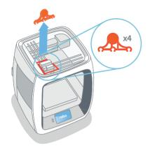
Remove the four orange protective gantry clips by pushing them over sideways with your thumb on the clip's round area (do not pull straight up).
