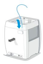
2. Insert filament feed tube into filament sensor block.
