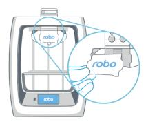
Magnetically attach extruder face plate (from accessories box) to extruder assembly.
