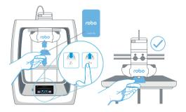
6. Slide the Z-Offset Tool between the nozzle and the print bed — tap the UP arrow on the touchscreen until you feel slight resistance against the Z-Offset Tool as you slide it between the nozzle and print bed.
